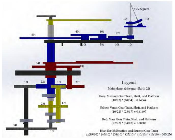
Figure 3: The gears, their teeth numbers, and how the gear train system is connected
